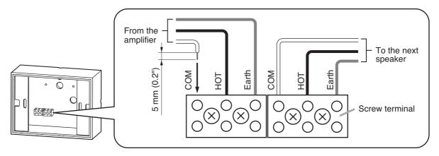
**3-2.** Insert the fasten s fitted at the ends of the HOT and COM cables from the screw terminals on the cabinet into the taps of the matching transformer on the speaker unit. Connect the COM cable to the transformer's COM tap, and the HOT cable to the desired transformer's input tap (Refer to the figure at right.)
