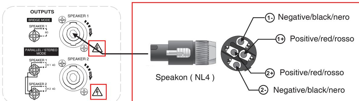
**NOTES:** The speaker connector can work from 4-16Ω in stereo or parallel model. It can work good from 8Ω to 16Ω in bridge mode.
