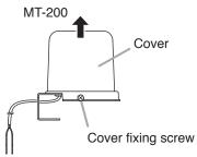
Step 2. Change the primary connection tap. The tap of the MT-200 is factory-preset to 167  $\Omega$ . Change the setting as required. To change the tap, reconnect the primary black cord
