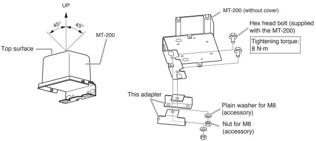
**Step 4.** Mount this adapter to the rear panel of the speaker module.
