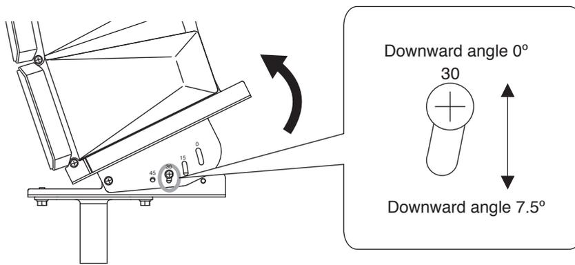
The figure shows the angle setting when in 30° mode. The downward angle can also be set similarly within the range of 0° to 7.5° when in 0° and 15° modes. However, the downward angle cannot be set when in 45° mode.
