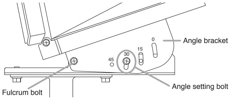
7-2. Lift the angle bracket, including the speaker with the fulcrum bolt as a fulcrum, so that the required downward angle can be obtained.
