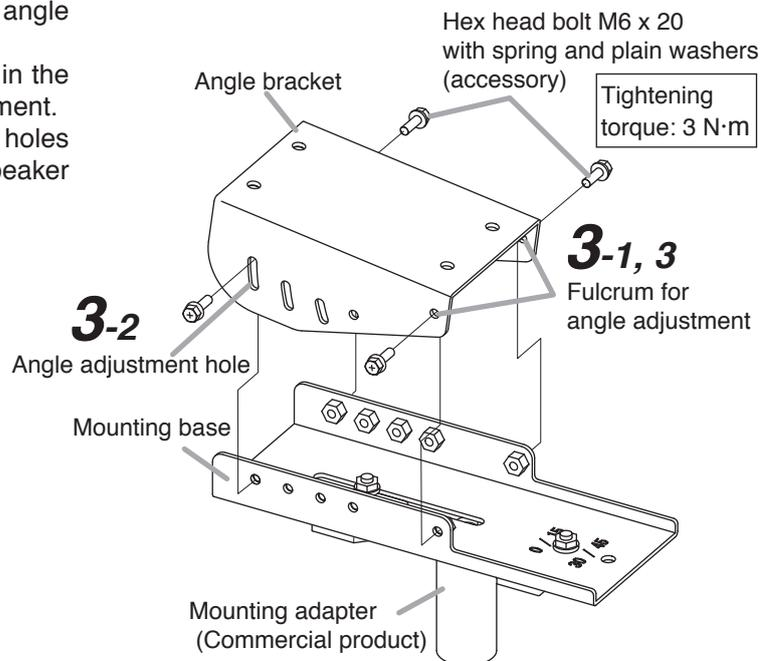
Fix the angle setting bolts in the positions corresponding to the set speaker directivity angle mode, as shown below:
