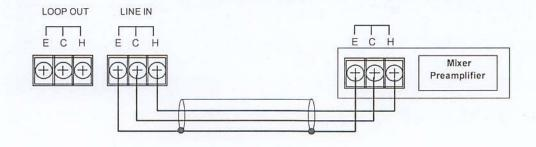
• Connection with the mixer preamplifier having the unbalanced type output. Please make the length of the cable less than several meters.
