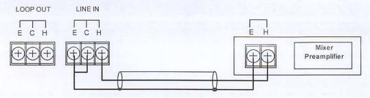
Speaker Line Input Connection It is connected to the High Impedance (70V /100V) speaker wiring of other amplifier.
