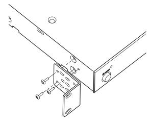
**Step 2.** Remove plastic plugs from top of the units, insert the joint bar into the case side slots, and fix it with screws (M3 x 6, black).
