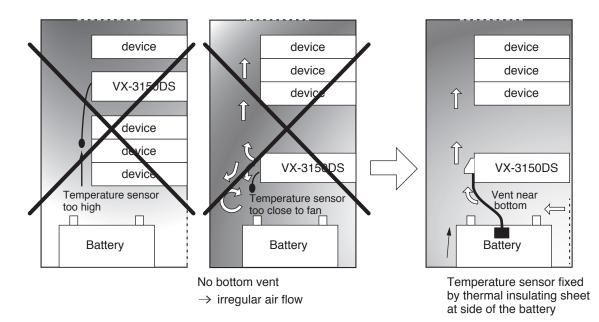
Figure 3: Incorrect and correct positioning of the temperature sensor in the cabinet rack
