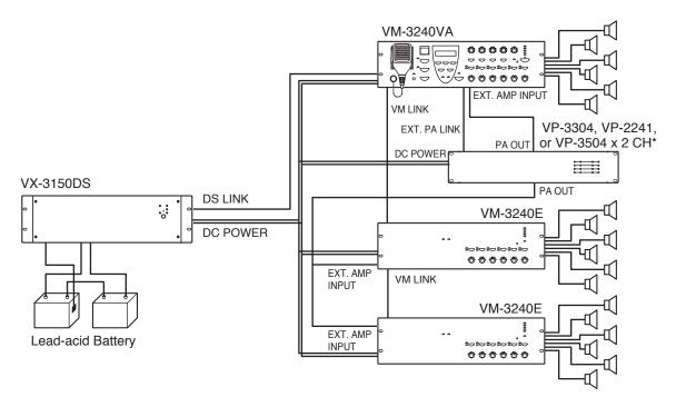
\* VP-3504 x 2 CH: That only 2 channels can be used when VP-3504 connect to VX-3150DS.
