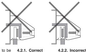
• Strip the cable end long enough (30 mm ± 5 mm) to be fully clamped. Otherwise, its outer jacket prevents the cable conductor from being tightly secured, causing poor contact.
