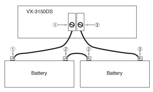
Touch the battery contacts and the screw tops of the battery connector of the VX-3150DS with the measuring tips as shown above.
