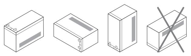
Figure 1: Permitted and forbidden installation positions of the battery
