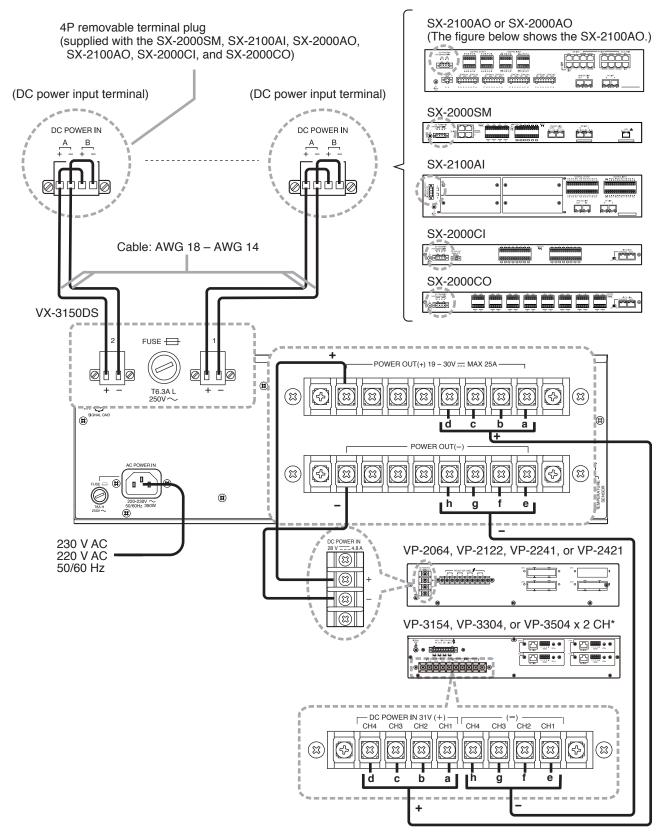
\* VP-3504 x 2 CH: That only 2 channels can be used when VP-3504 connect to VX-3150DS.
