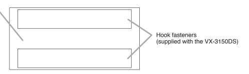
When replacing the batteries, 4 each of fastener hooks and loops, and a thermal insulating sheet listed below are also required. Consult your nearest TOA dealer on how you can obtain them.
