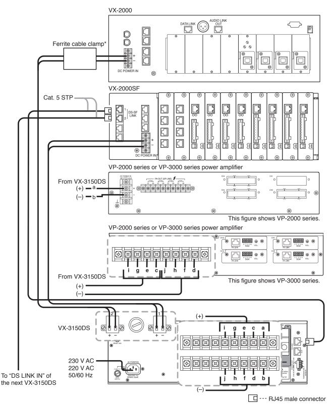
\* Ferrite Cable Clamp Attachment (For VX-2000 only) To reduce electromagnetic noise, place the supplied ferrite cable clamp over the DC power cable at a position within 20 cm from the VX-2000's DC POWER IN terminal.
