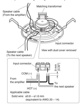
3-2. Change the input impedance as needed. The speaker's input is factory-preset to 1.7 k $\Omega$ . When changing the input impedance, detach the black wire connected to the matching transformer,
