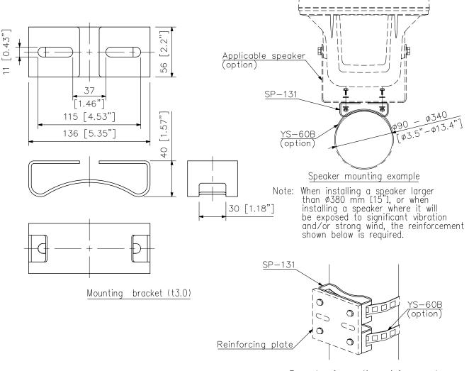
Example of mounting reinforcement
